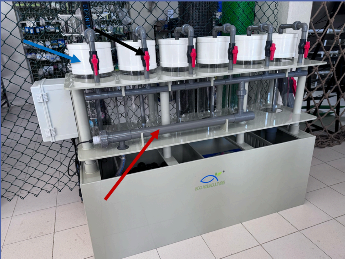
Figure 10: The fry incubation unit. The components include the incubation jars (blue arrow) in which fertilized eggs are placed; inlet pipes (black arrow) through which water flows into the jars; UV light section (red arrow) through which water flows and is treated in the process; outlet pipe (yellow arrow) that brings back overflow water from the jars into the tank reservoir (green arrow) (Image by Victor Omondi).
