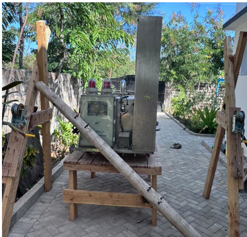
Figure 4: The FTU lift which uses two manual winches to lift the FTU up during loading and offloading onto the pickup
